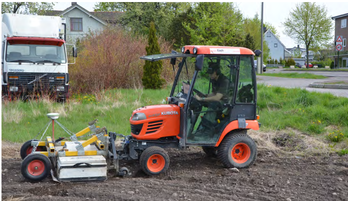
Figure 5: The 16 channel 400 MHz MALÅ Imaging Radar Array (MIRA).
