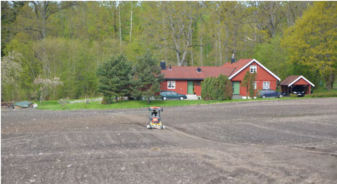
Figure 2: High-resolution GPR prospection in Horten / Granly skole using the MALÅ Imaging Radar Array.
