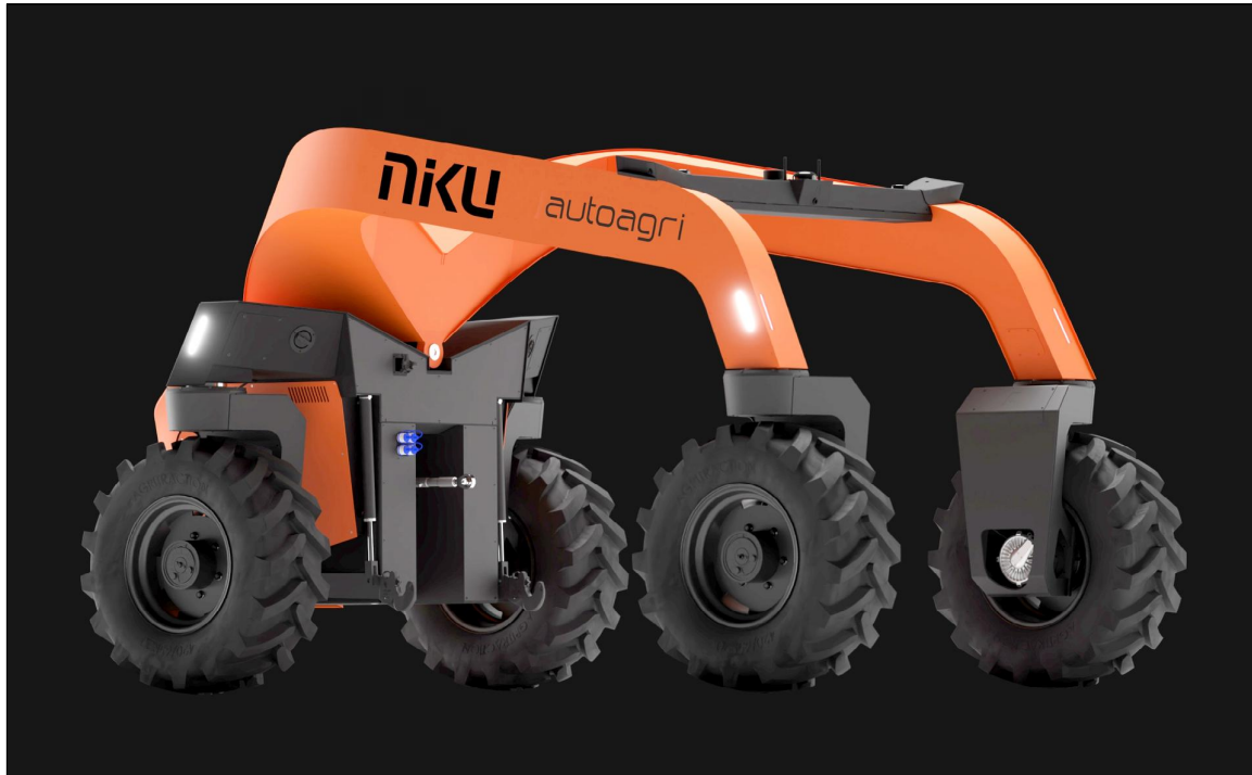
Fig. 1: Computer rendering of the AutoAgri ICS20E implement carrier to be used in the presented project. The MIRA HDR system will be mounted centrally between the wheels.
