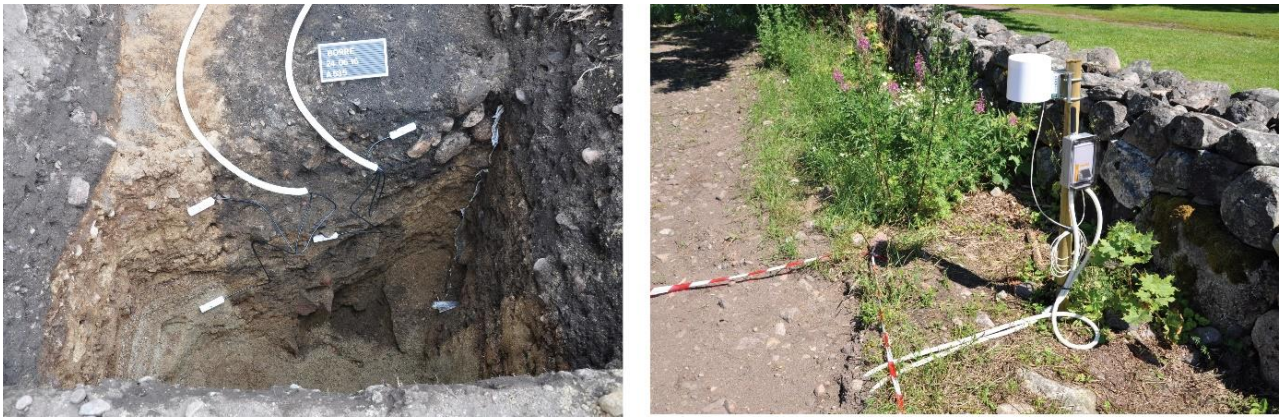
Figure 4. Monitoring station 1 with in situ measurements of VWC, BEC and ground temperature ( left ) as well as precipitation using a high precision rain gauge. Data were recorded by a remotely accessible datalogger ( right ).
