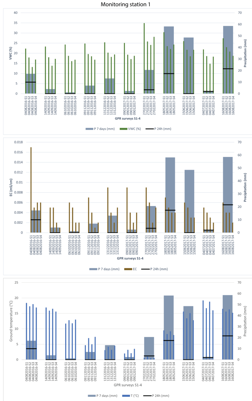
Figure 12. The comparison chart displaying the values measured for the VWC, BEC and ground temperature for sensors S1–S4 at monitoring station 1 during each of the GPR surveys. Precipitation rates are displayed for the week (blue bar) and 24 h (black line) prior to respective survey dates.
