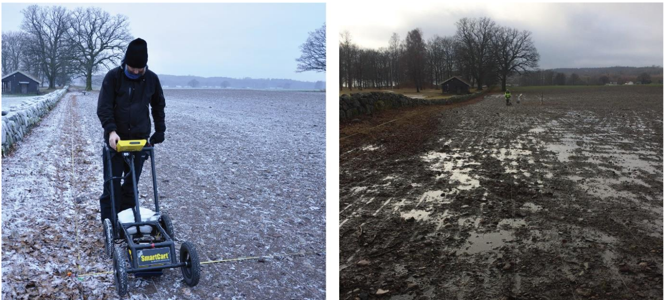
Figure 14. Pictures taken during the GPR surveys in January 2017 under very cold and dry conditions ( left ), and in February 2017 when the partially frozen topsoil began to thaw ( right ).
