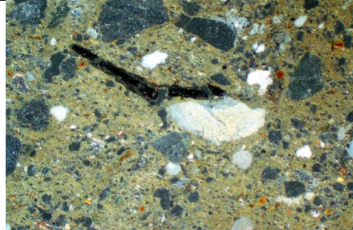
Fig. 61; As Fig 60, under OIL; charcoal is often included in mortars because this is relict of lime making.
