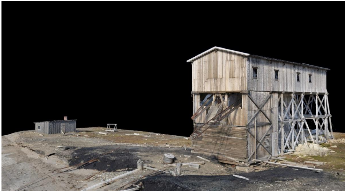
Figure 5. Textured 3D mesh model of the cultural heritage objects no. 1–7. The photogrammetric model was created using a combination of 3D laser scans and a series of single images. Geometry of the model is mainly based on laser scans, and photorealistic colour is derived from single images.
