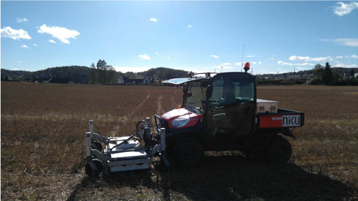
Figure 7: MIRA 3 at Auli. The MIRA box is mounted in front of a Kubota RTV. The RTK-GPS is mounted on top of the MIRA box. Foto: Manuel Gabler / NIKU.
