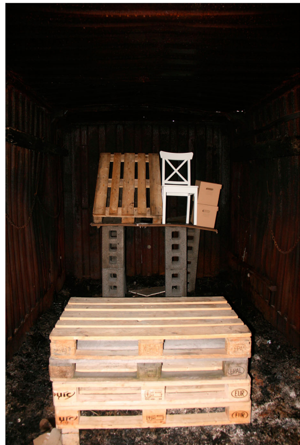
Figure 3. Set-up before covering the items and before igniting the fire using the wooden pallets stacked in front.
