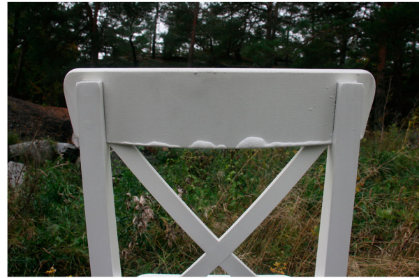
Figure 7. Example of damage after the water test: water damage on painted wooden chair. Minimal covering with gaps on the side allowed humidity to get inside and react, causing the material to swell.
