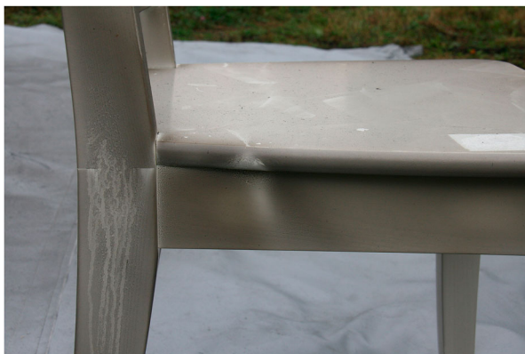
Figure 6. Example of damage after the fire test: soot on painted wooden chair. Minimal covering with gaps on the side allowed soot to get inside.
