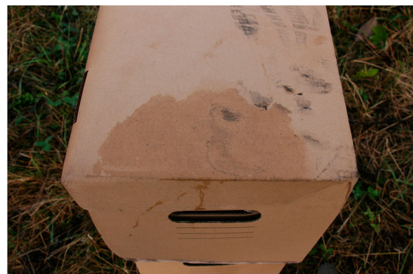
Figure 8. Another example of damages caused by water on the cardboard box. The seams on some of the covers resulted in wet cardboard boxes underneath the cover.
