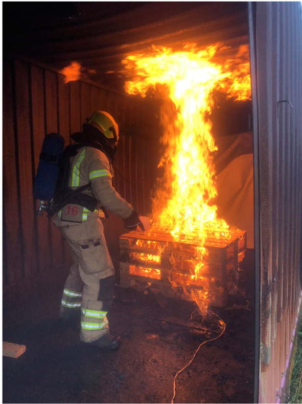
Figure 5. Igniting the stacked pallets for fire test.
