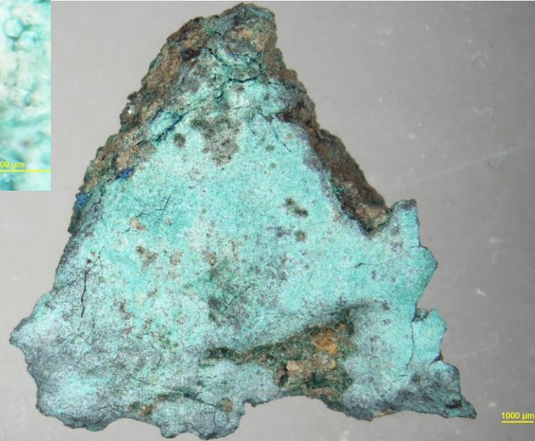
Figure 18. Micrographs of copper fragment from SL4179. Malachite (green color) covers most of the surface, although some azurite (blue) is also present.
