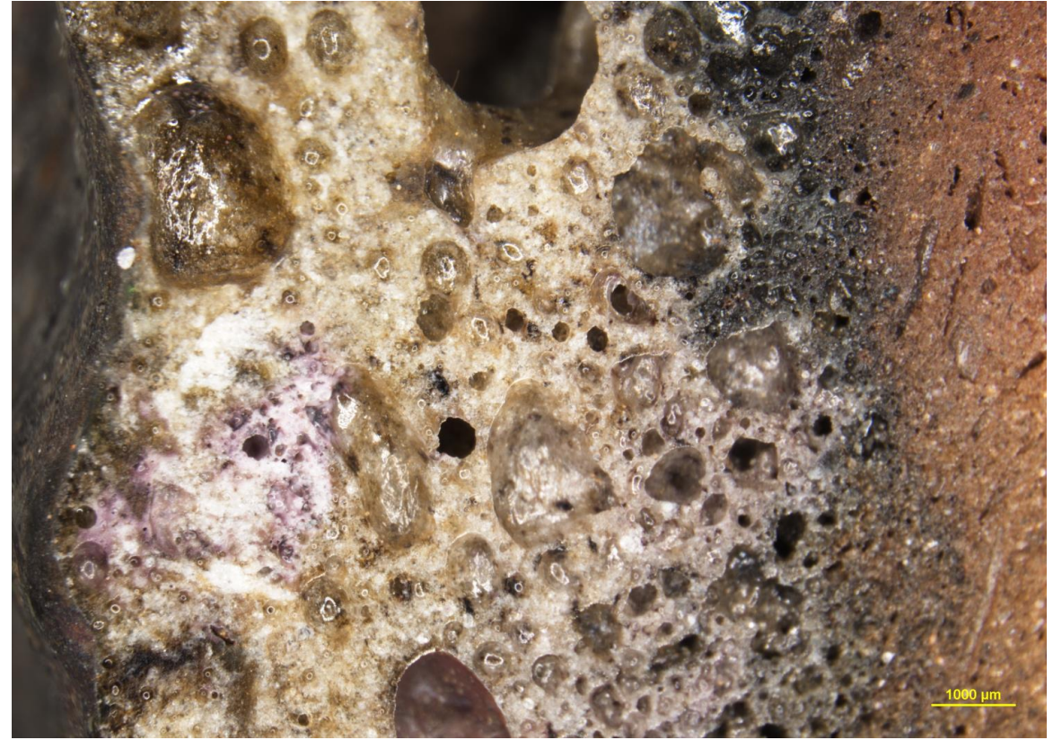
Figure 7. Cross-sectional view of vitrified clay materials from SL4729.
