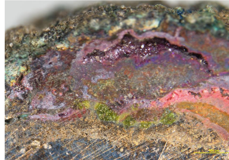
Figure 15. Micrographs, taken with a stereomicroscope, illustrating the various layers of corrosion products visible on the metallic nodule of leaded bronze from SL3848. Cuprite (red), copper chloride (brownish), and malachite/copper oxychlorides (green) are all visible in cross-section. The sampled area can be seen on the left.
