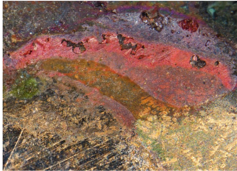
Figure 15. Micrographs, taken with a stereomicroscope, illustrating the various layers of corrosion products visible on the metallic nodule of leaded bronze from SL3848. Cuprite (red), copper chloride (brownish), and malachite/copper oxychlorides (green) are all visible in cross-section. The sampled area can be seen on the left.
