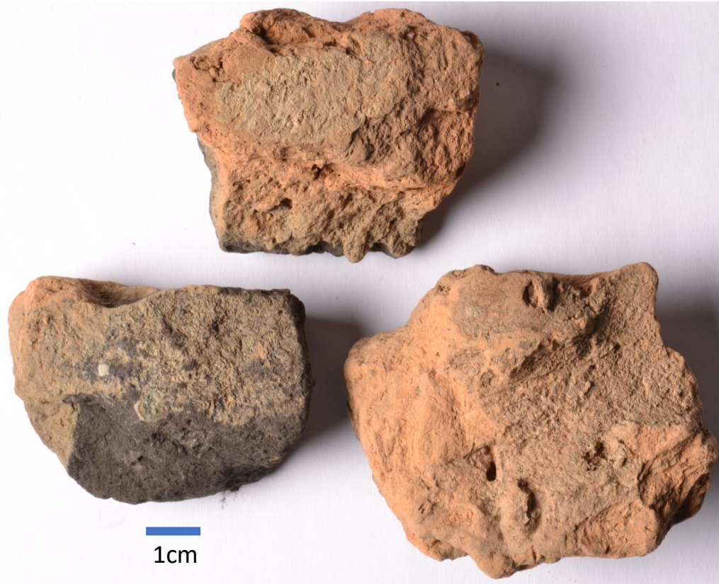
Figure 1. Red clay materials from SL4729, outer side (left) and inner side (right). The low degree of vitrification on the inner surface implies exposure to a relatively low temperature.
