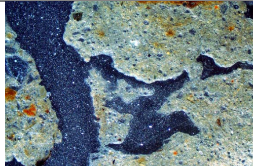
Fig. 3: As Fig 2, under oblique incident light (OIL). Note generally iron poor fine fabric.
