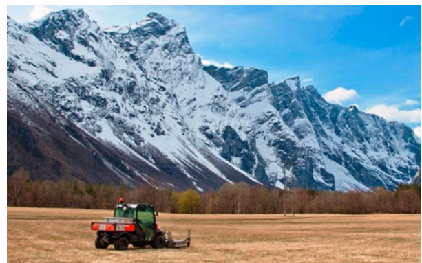
Figure 1: NIKUs motorized MALÅ MIRA system applied at Marstein, Møre and Romsdal county, Norway.
