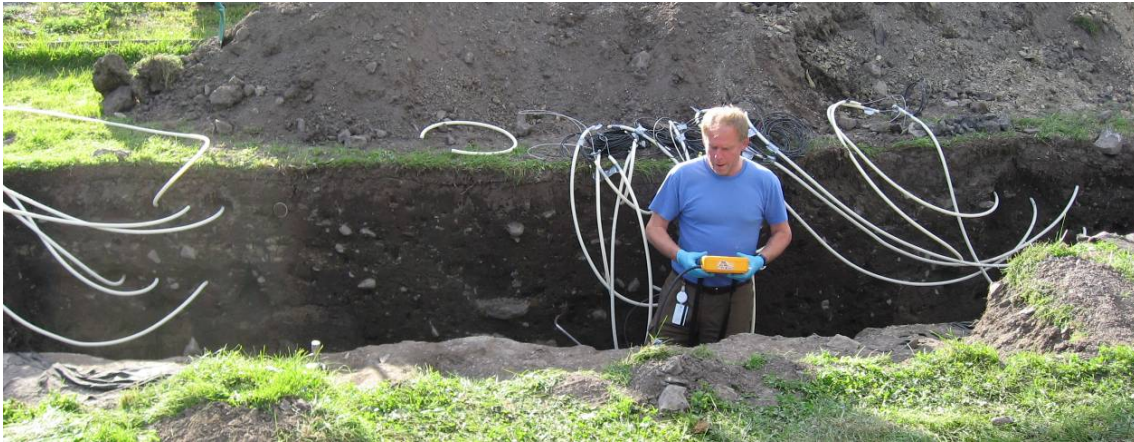
Figure 40 Section in trench G, Åker 2007, with soil probes installed. VVM/NIKU.
