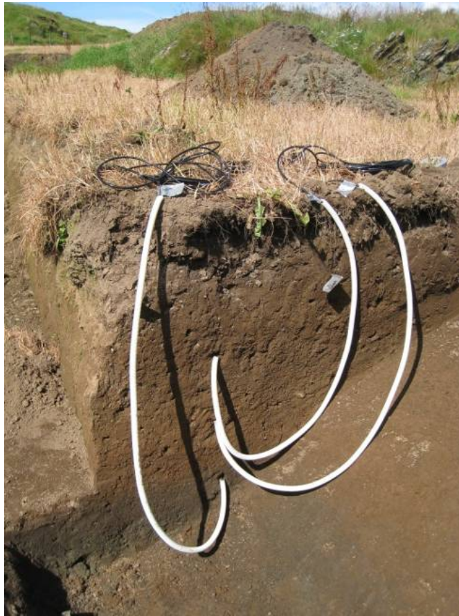
Figure 51 Installed probes in the cultivation area. VVM/NIKU.
