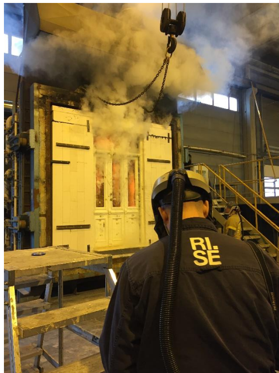
Figure 2-6 Fire resistance test. Glass panes have broken, smoke and flames are visible. Photo: B. Wedvik, NIKU 2019.
