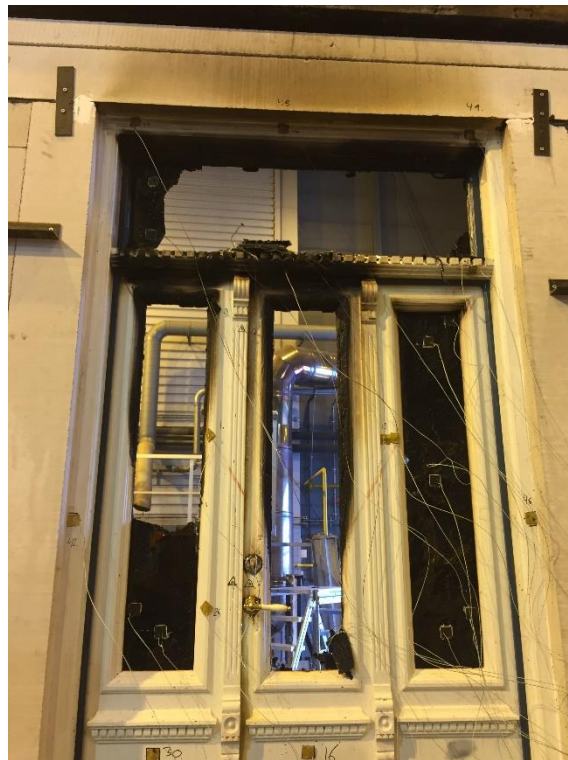
Figure 2-7 Fire resistance test. Test is ended. All glass panes are broken. Photo: B. Wedvik, NIKU 2019.
