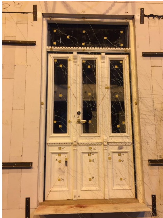
Figure 2-5 Fire resistance test set-up for old stairwell door. Thermocouples are shown attached to door, registering the temperatures on the unexposed side. Photo: B. Wedvik, NIKU 2019.
