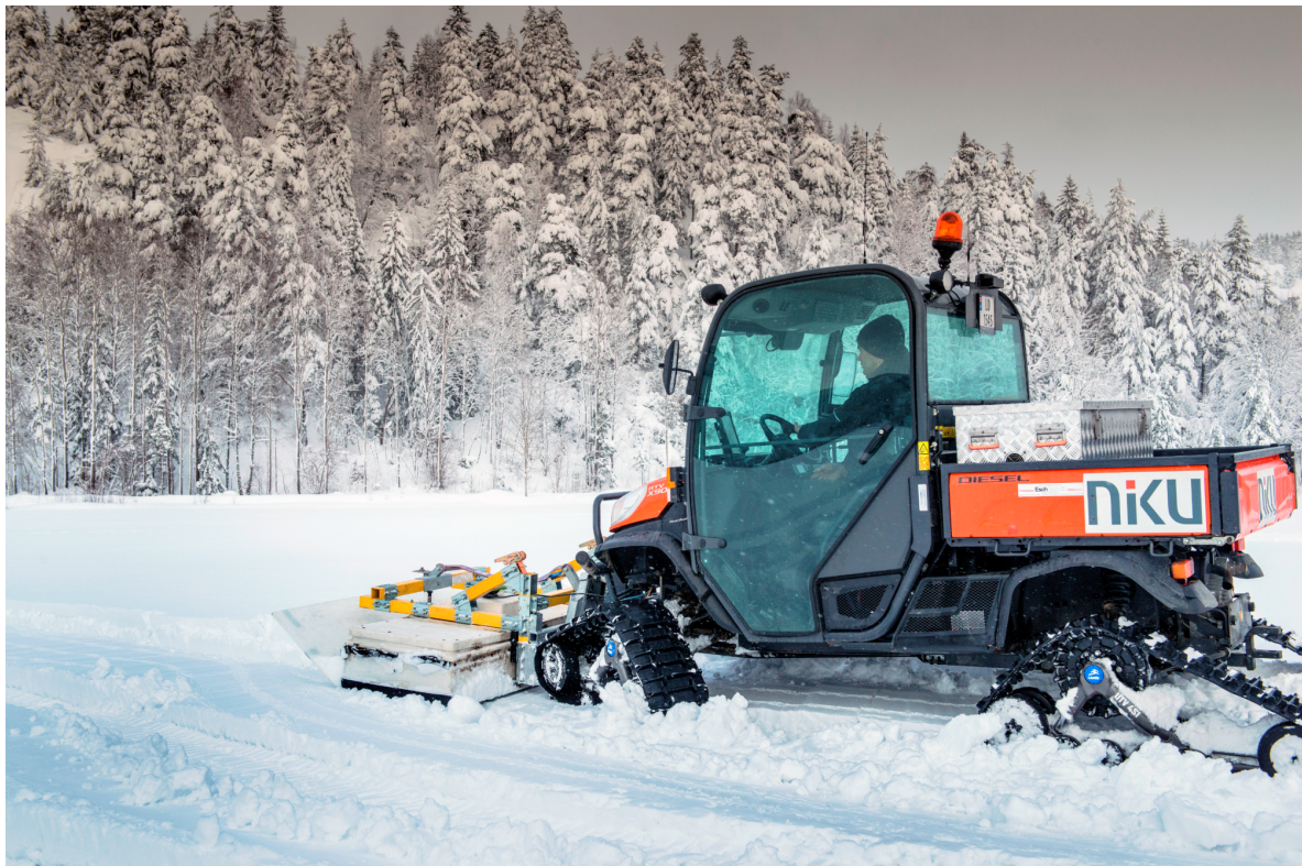
Figure 1. NIKU's 16-channel MIRA system configured for winter survey with snow crawler belts at Odberg in Lågendalen. The GPR antenna array is housed in the white box placed on a large skid plate in front of the Kubota Rough Terrain Vehicle. Photo: Erich Nau.
