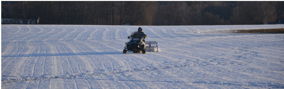
Figure 2. GPR survey with a 500 MHz SPIDAR system with 25 cross-line channel spacing at Borre. Photo: Roland Filzwieser.
