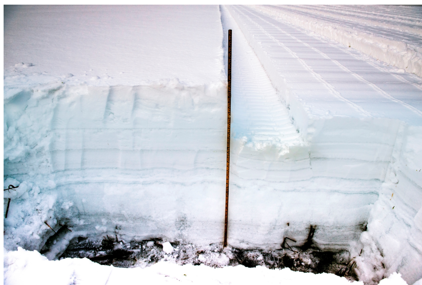
Figure 4. 100 cm thick snow cover at Odberg during the GPR measurements in February 2018. Note the compacted snow caused by the snow crawlers to the right of the yard stick. Photo: Erich Nau.
