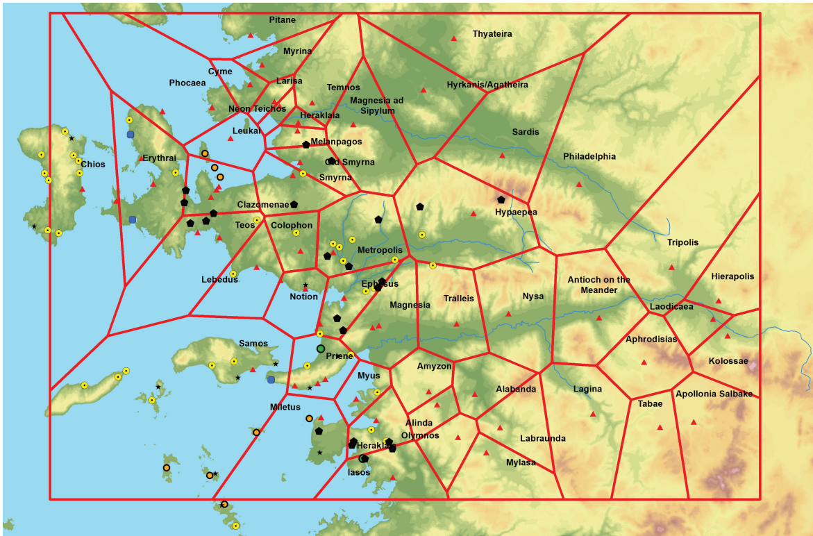
Figure 8. Illustration showing algorithmic generated Thiessen polygons.
