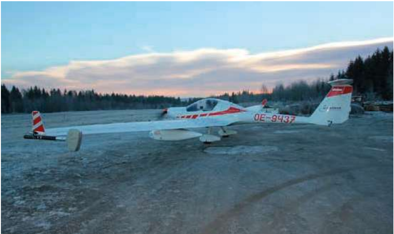
Figure 7. A light aircraft from Airborne Technologies with magnetometer sensors mounted on the wing tips and ready for take-off. Photo: NIKU
