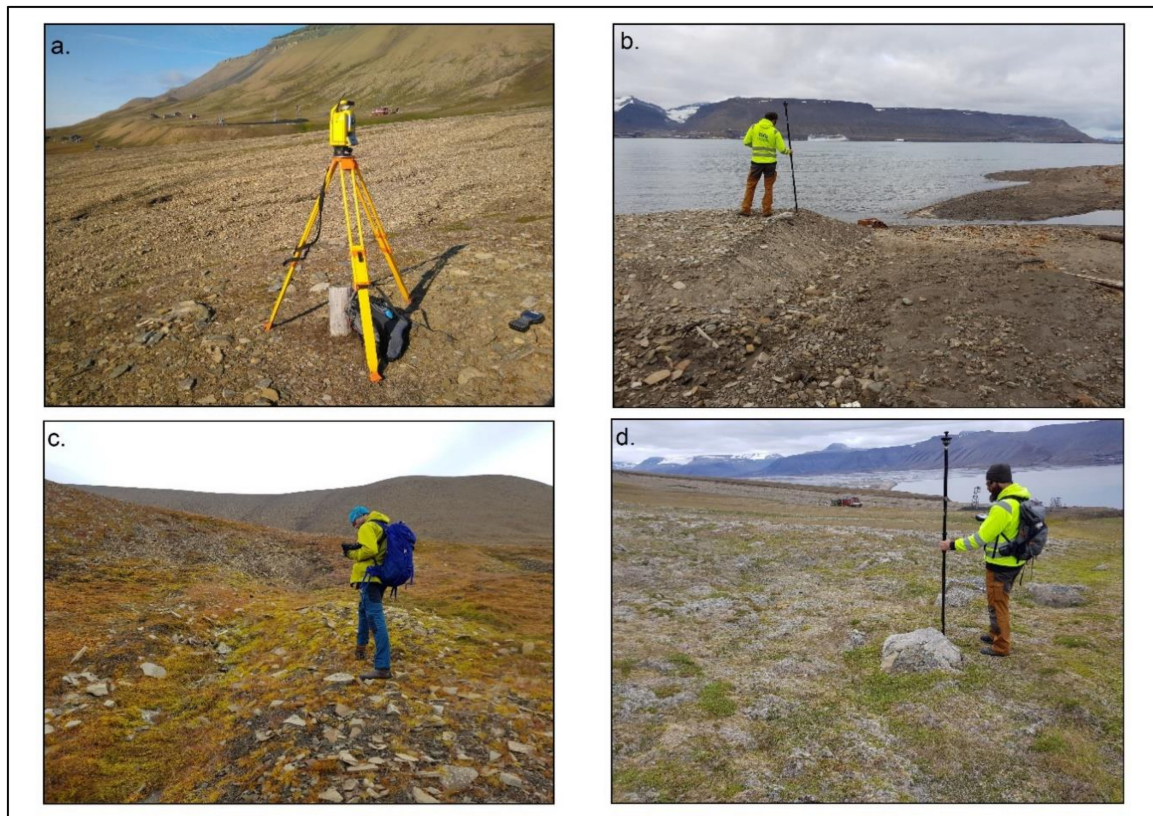
Figure 5. (a) Total station and controller on one of the fixed points; (b) Coastline survey; (c) Geological mapping of the upper area of Hiorthhamn; (d) Survey of surface soil movements.
