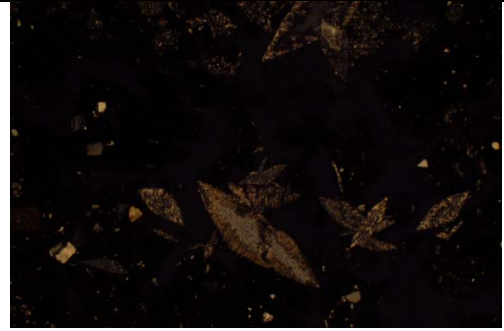
Fig. 20: As Fig 19, under crossed polarised light (XPL), with 1st order grey birefringent prismatic gypsum ( \text{CaSO}_4 \cdot 2\text{H}_2\text{O} ).
